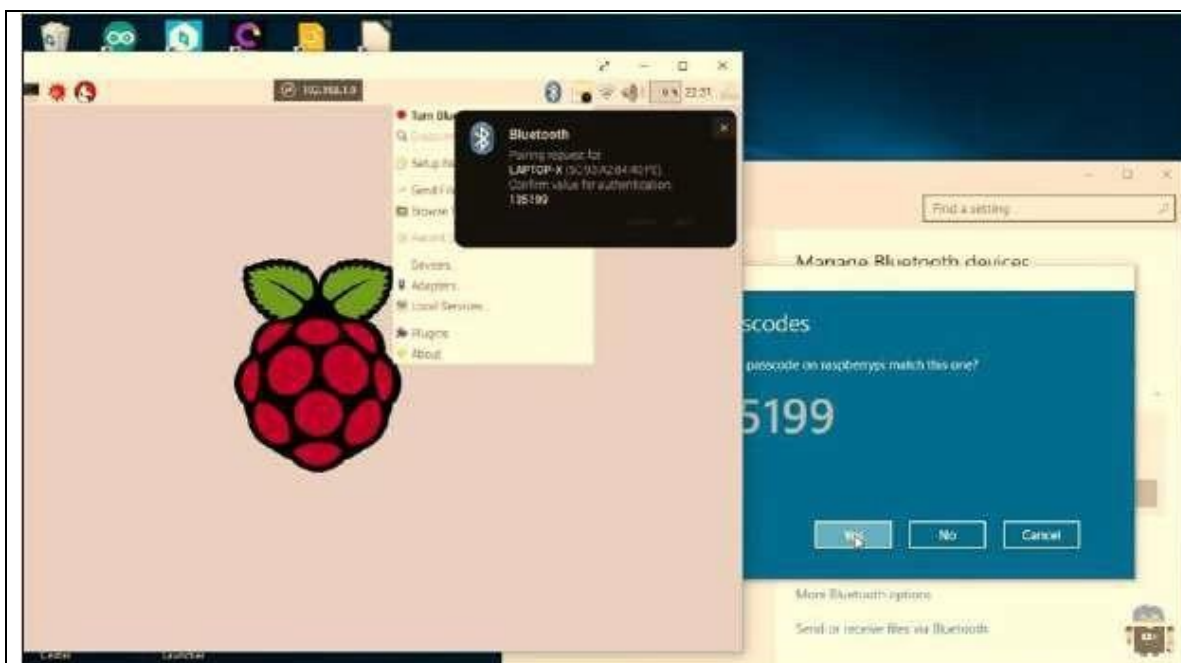
Fig. 4.20: Checking the passcodes
