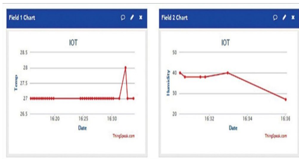
Fig.10.5: Graphical view of humidity and temperature on Thing Speak platform
