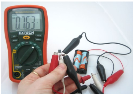
Fig. 6.10: TMP36 sensor testing at room temperature
