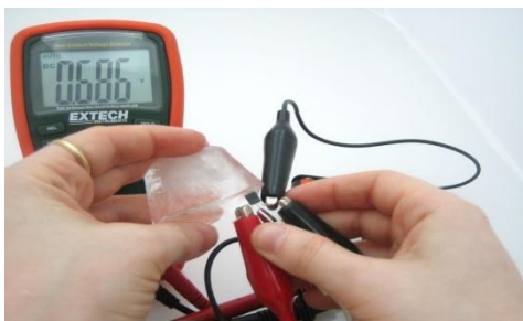
Fig. 6.12: TMP36 sensor testing at low temperature
