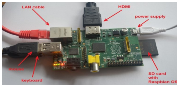
Fig.1.23: Connection set up of board
