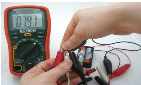
Fig. 6.11: TMP36 sensor testing at high temperature
