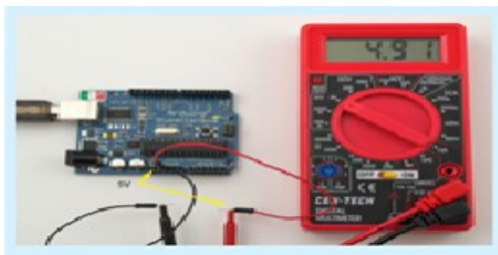
Fig. 7.8: Change power source and measure Vin in Arduino board
