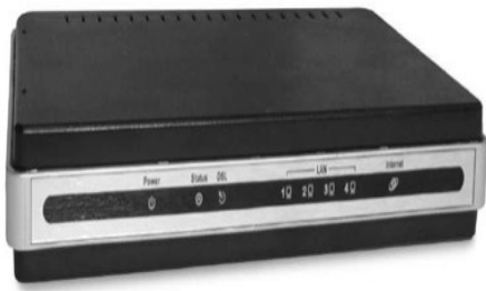
Fig. 3.12: Router LED indicator
