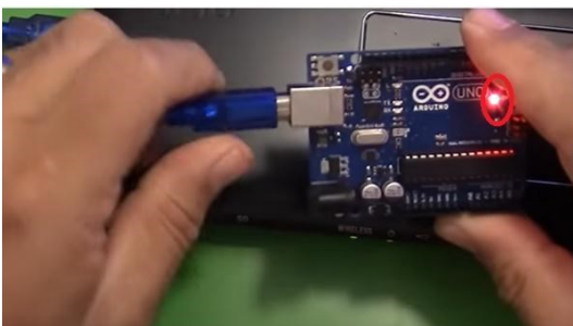
Fig.1.17: LED blinking on the Arduino board after connecting the USB cable
